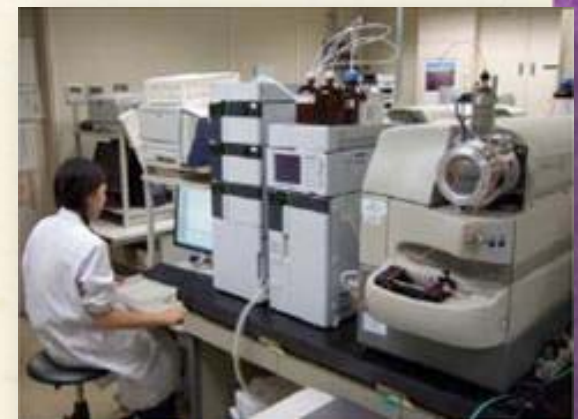
Analysis using High-performance liquid chromatograph-mass spectrometer
