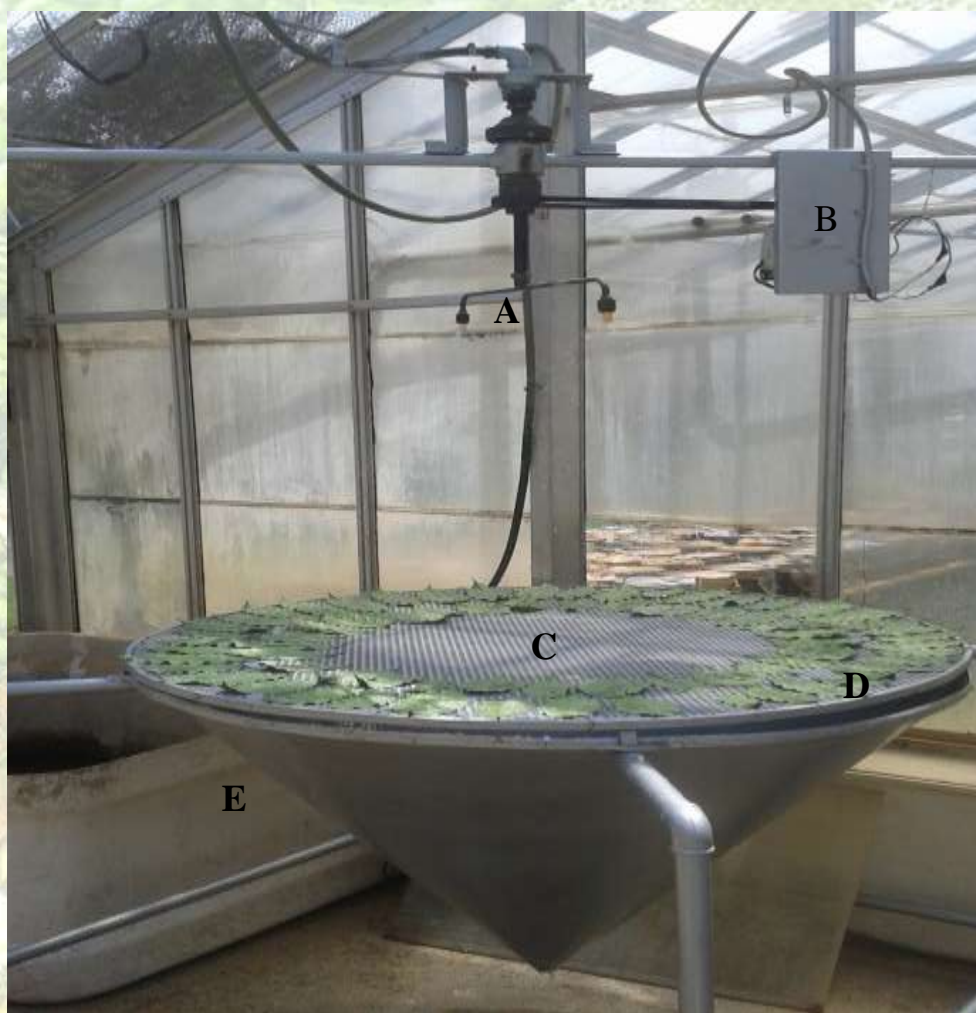
Figure 1. Rain simulator used in the experiment. (A) Rain simulation nozzles. (B) Control and adjust nozzle speed. (C) Spray table. (D) Coffee leaves. (E) Water reservoir and pressure control.
